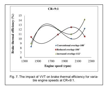
The percentage increasing of brake thermal efficiency at CR=9 than CR=7 by (4.034 % for Conv. overlap=108°), (7.229 % for
