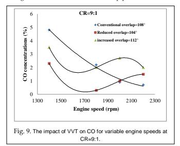
At (overlap=112°) the CO concentrations decreased due to the combustion improvement. Also, the (IEGR) effects to decrease the CO emissions, with the method of Late Exhaust Valve Close (LEVC). A certain amount of exhaust gas is allowed to
