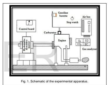
The hydraulic brake (or hydraulic dynamometer) used to measure the torque output from the engine by friction fluid. Water used as the friction fluid. To measure dynamometer load a hanging weight balance is used to overcome the tilt in the torque arm to keep it in the horizontal position, the following equation used to calculate the torque:
